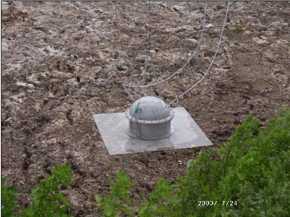
**Figure 13: Close-up of flux chamber at point 2.**
