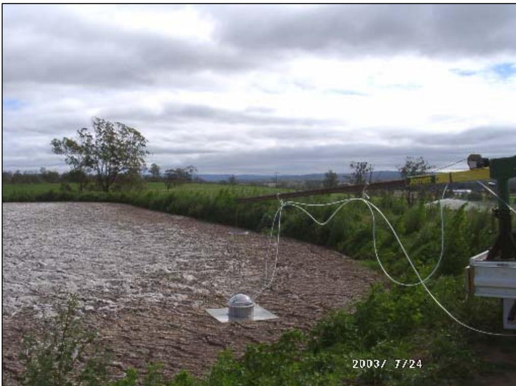
**Figure 12: USEPA flux chamber at point 2 on the primary lagoon**
