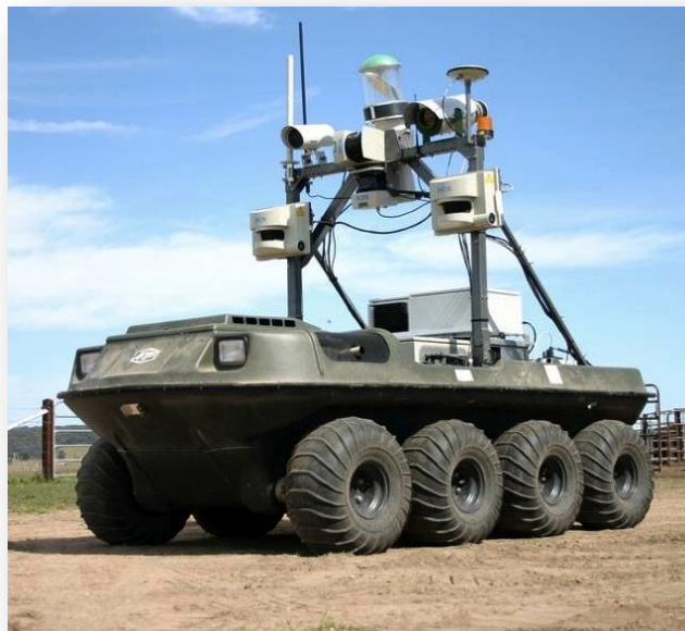
Figure 35: the Argo autonomous vehicle was developed at the ACFR with the aim of building an intelligent multi-purpose platform that could be used in unstructured and undulating terrain. The system is equipped with various laser, radar and thermal sensors, and is capable of long distance and beyond line-of-sight operation.
