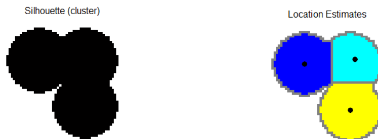
Figure 23: The goal of the cluster delineation algorithm is to split a classified silhouette of a cluster of trees into estimates of the locations of the tree crowns that compose it.
