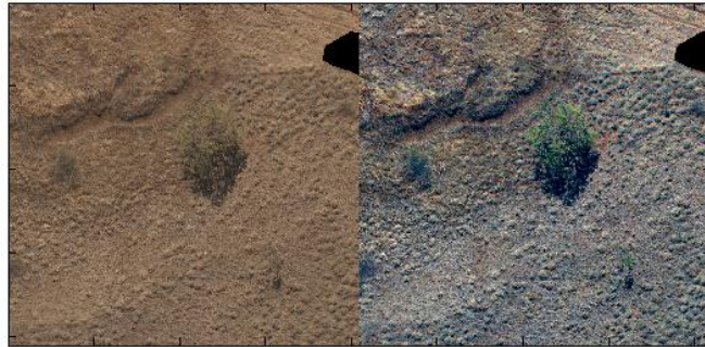
Figure 7: An example of the pixel spectral whitening that is applied as a pre-processing step before classification to assist both in feature extraction and in the supervised human interpretation of the imagery.
