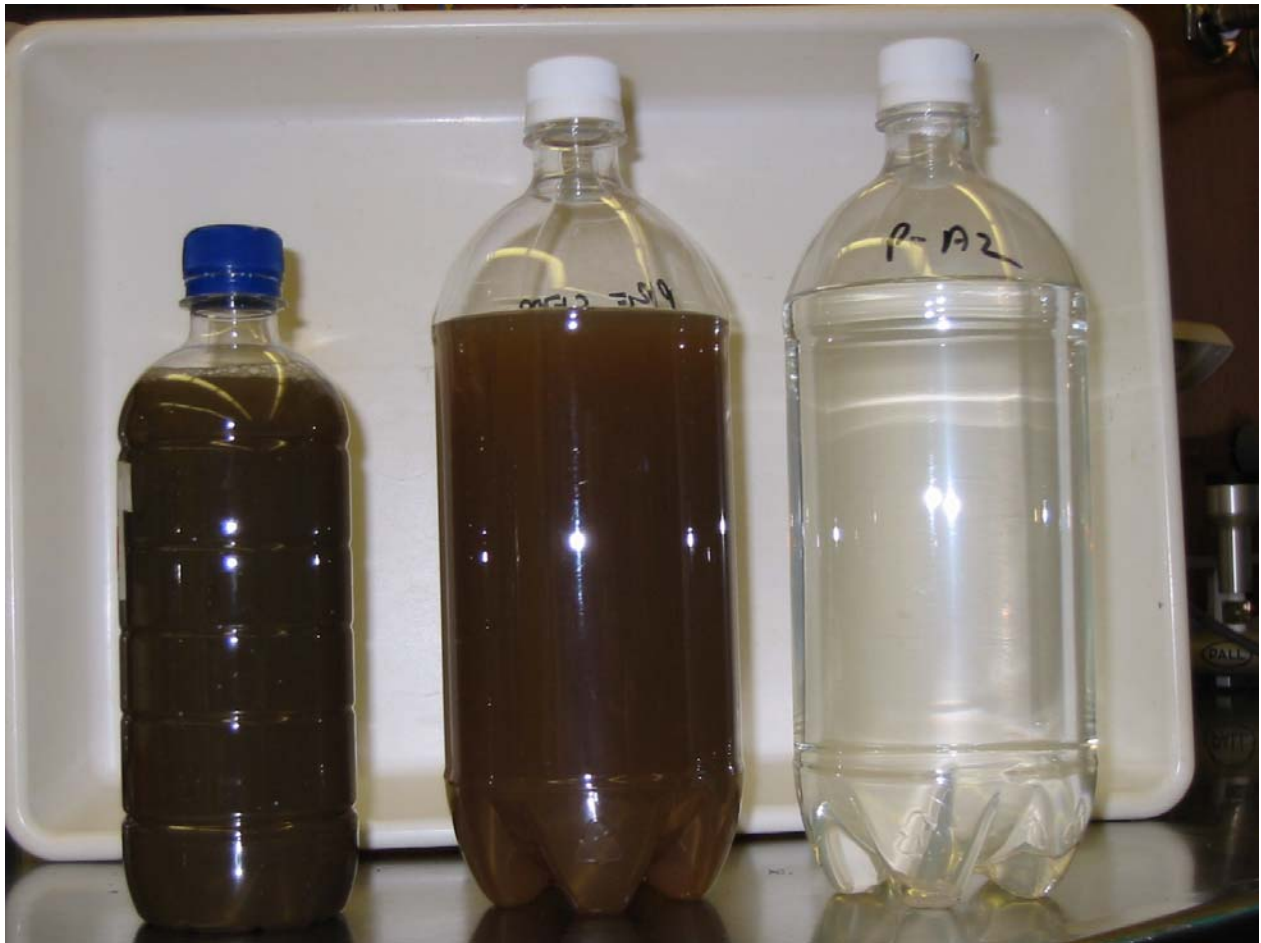
Figure 2: Comparison of waste water influent, treated waste water and the product water
