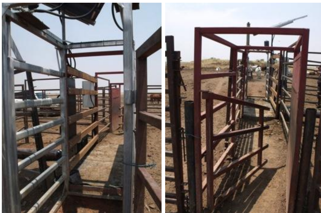
Figure 4 - WoW platform showing the different components including: the weigh platform, crush, RFID panel reader and data logger and drafting gate (left). Front entrance to remote WoW system operating on a station in the NT (right). The spear gate prevents animals from returning back over the platform and forces them to use an alternative exit.
