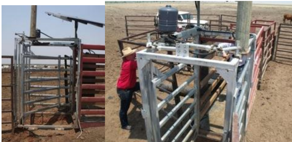
Figure 5 - Auto-drafting gate on the front of WoW platform. The auto-drafting gate swings towards the viewer allowing animals to be drafted either straight ahead or towards the viewer. This auto-drafter uses compressed air to operate gas struts, which change the gate position.
