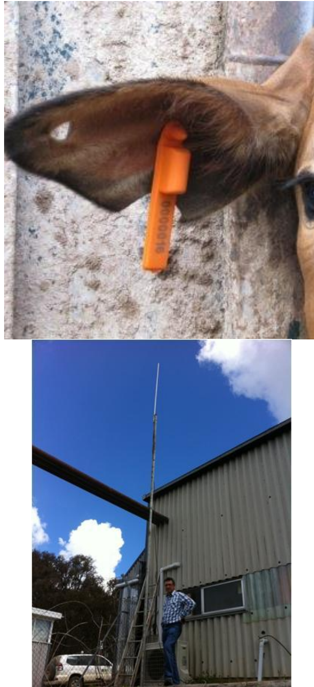
Figure 7 - A Taggle system ear tag that periodically emits a radio signal that is received by static towers enabling triangulation of position (above) and a Taggle System receiving antenna on a simple tower (below).
