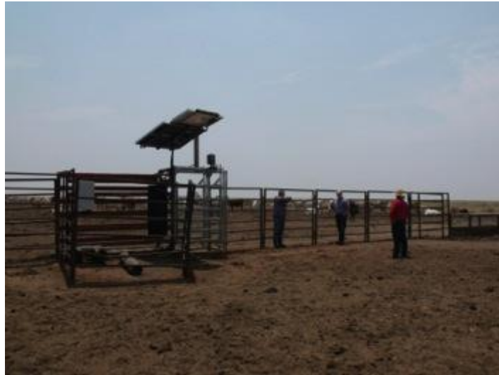
Figure 6 - This auto-drafter at station in the NT enables cattle to be drafted into one of two sets of yards for differential supplementation.
