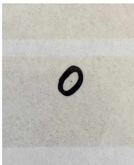
Fig. 2 Enlarged image of a typical contaminating particle visualised on tape samples from linerless carton blanks.
