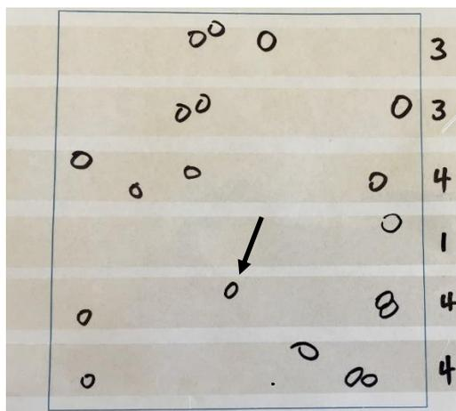
Fig. 1 Pressure sensitive tape technique for the determination of surface cleanliness. Tape samples from six (6) carton blanks appear as horizontal shaded zones. Circled areas are visible contaminating particles with the total number of particles per 25 cm<sup>2</sup> shown on the right. Arrow shows particle enlarged in Fig. 2.
