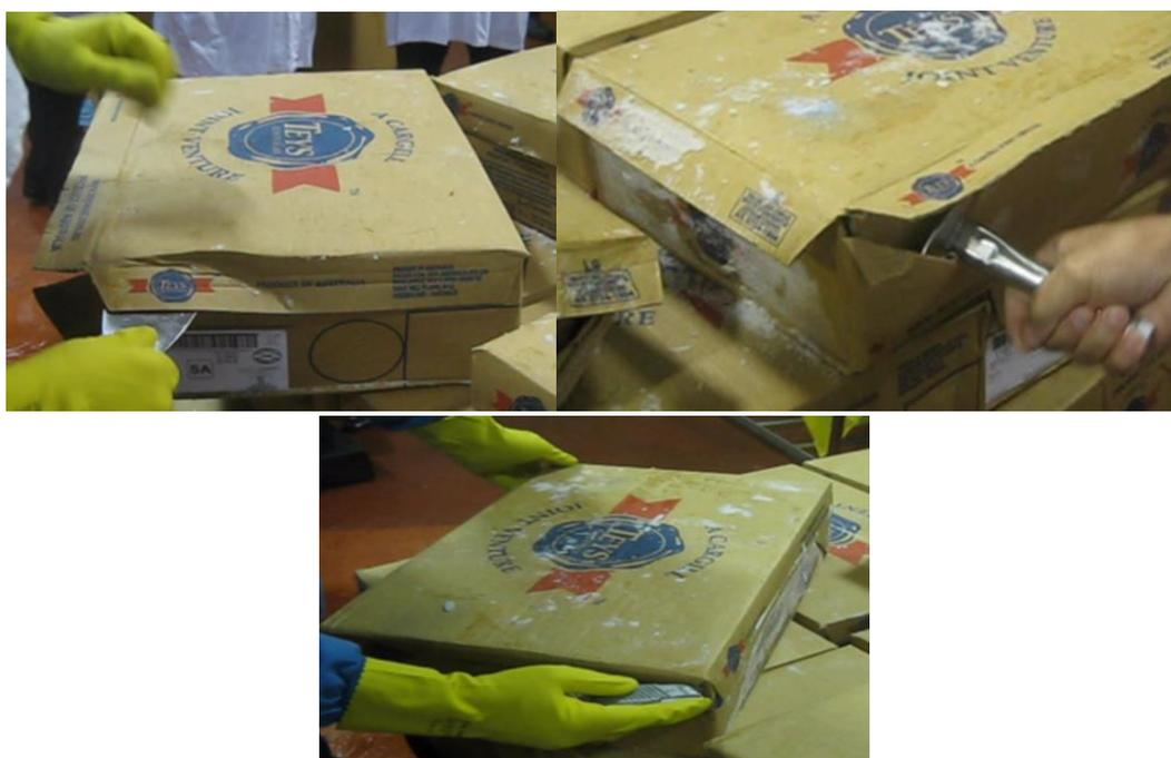
Fig. 8 Opening of linerless cartons after tempering using a commercially available spatula (a), purpose-built tool (b) or knife (c).
