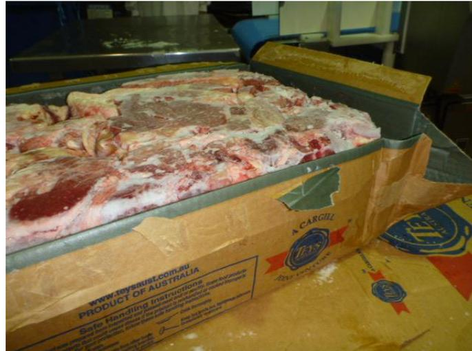
Fig. 5 Carton de-lidded showing delamination of the liner on the where it contacted glue on the carton lid.
