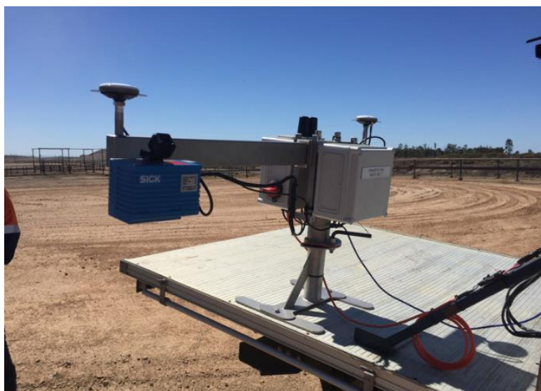
Figure 1 Automated bunk scanner developed by Manabotix Pty. Ltd and Meat & Livestock Australia Limited.
