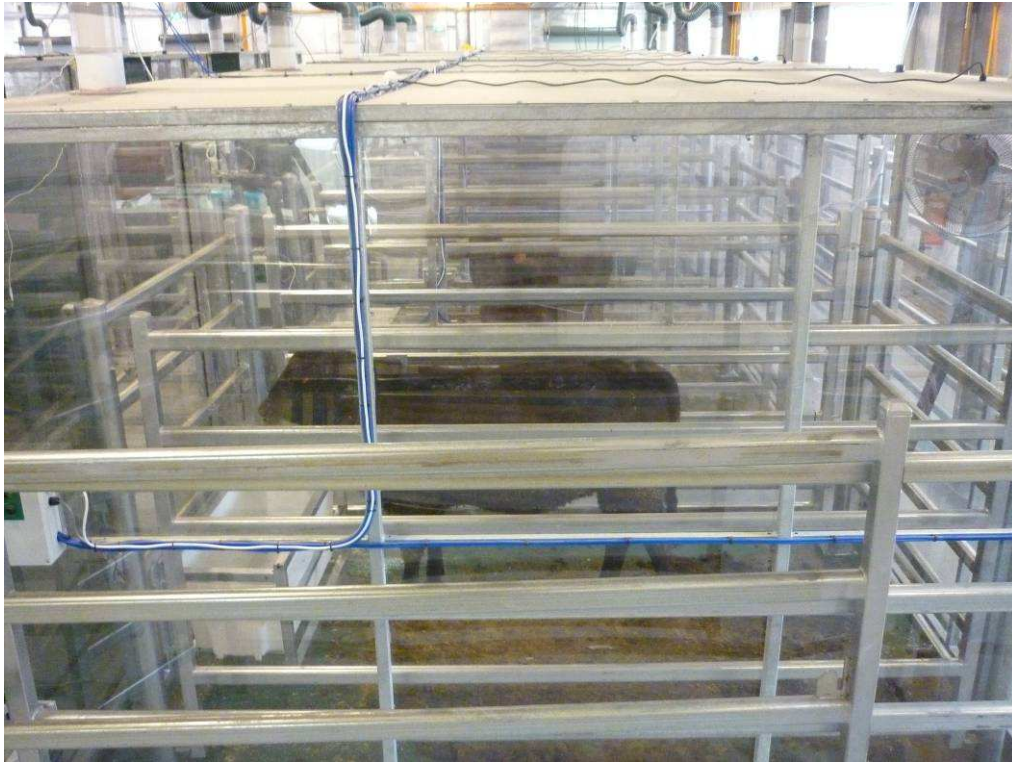
Angus bull inside methane measurement chamber with feed and water provided.
