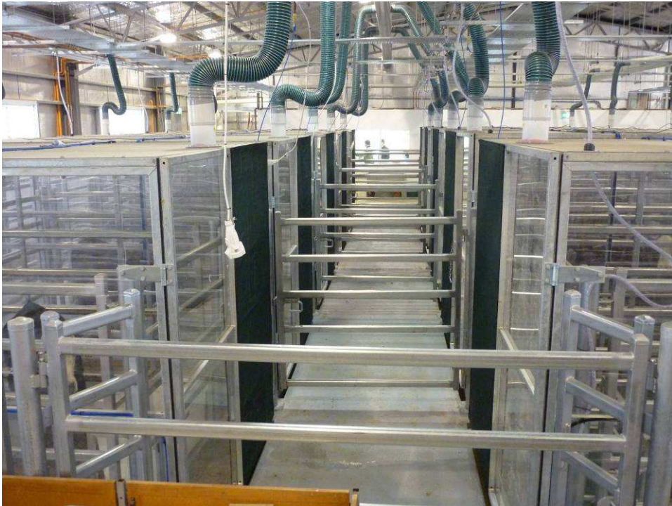
Methane chambers: two rows of five chambers with gas sample ducting.
