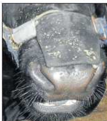
The animal's halter is fitted with a leather nose patch that holds the gas collection tubes above the nostrils, allowing continuous sampling of exhaled gas. (Photo: Reg Woodgate.)
