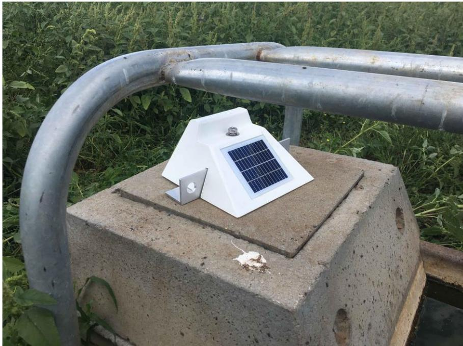
Figure 2. Wireless trough sensor v1 surrounded by vegetation - Windy Station
