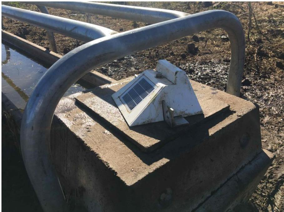
Figure 3. Wireless trough sensor v1 after 7 months in the field - Windy Station
