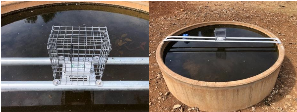
Figure 7: Modified Water trough sensor
