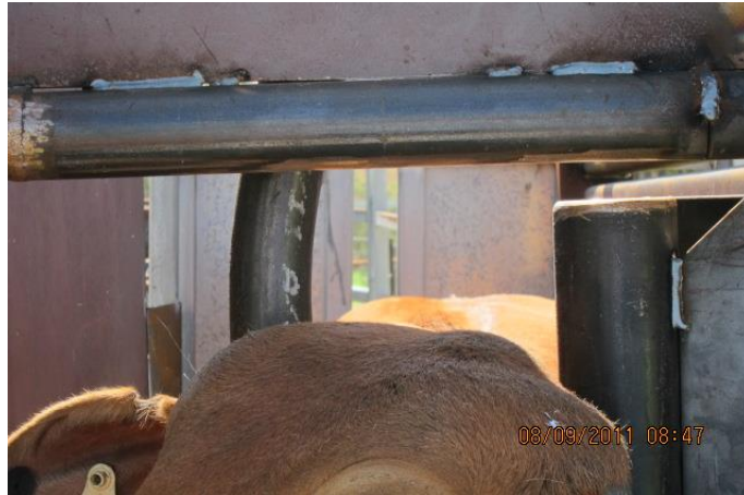
Figure 8 -Shows the gap between the sub structure of the box and the head bale that allows for vertical head movement. First live trial 16 September 2011.
