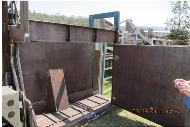
Figure 6 - The hinged door that releases the head bale and allows the animal to exit the restraining box. First live trial 16 September 2011.
