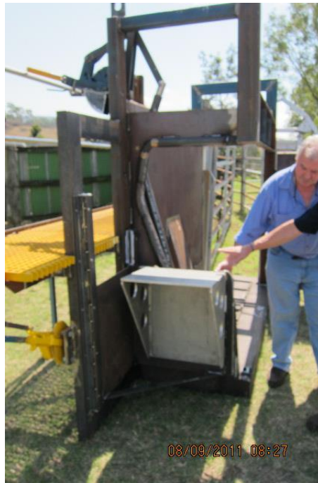
Figure 7 - Head bale lever in the open position. First live trial 16 September 2011.
