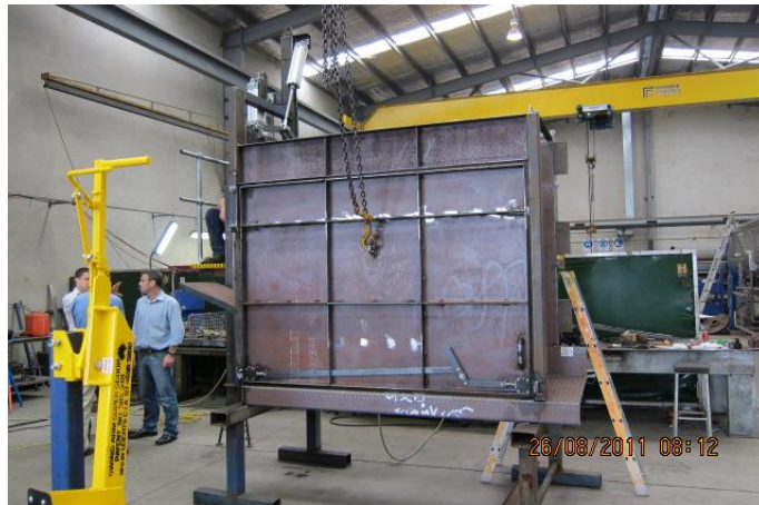
Figure 5 - Note the block and tackle located in the centre of the restraining box which would be employed to open the door. Site visit to G & B Stainless 26 August 2011.
