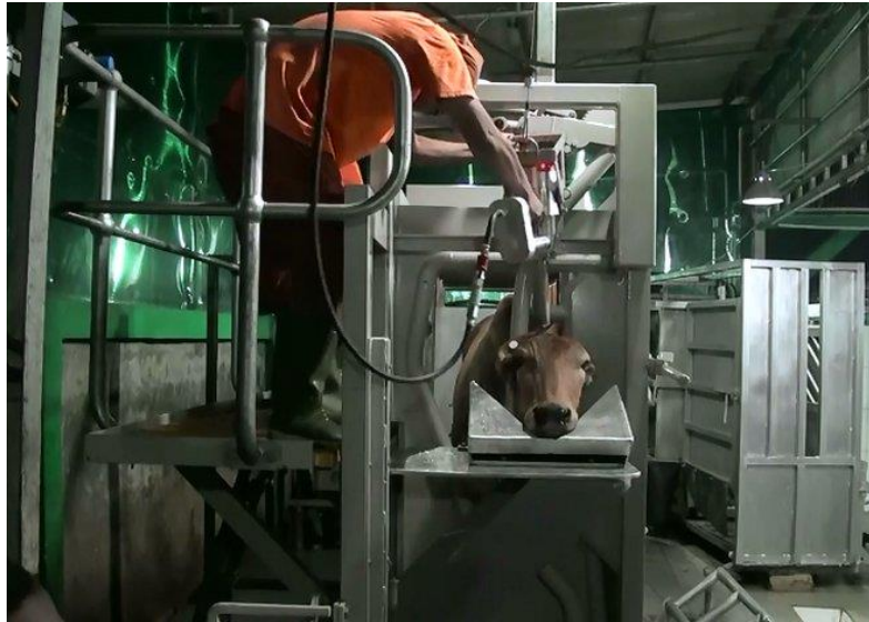
Figure 11 - The concave head restraint plate positioned the animal's head squarely for the stun application. Prototype installed and operational in Indonesia.
