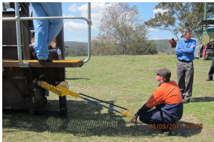
Figure 10 - Head lift ratchet lever fully extended but not properly engaging the head of the animal.
