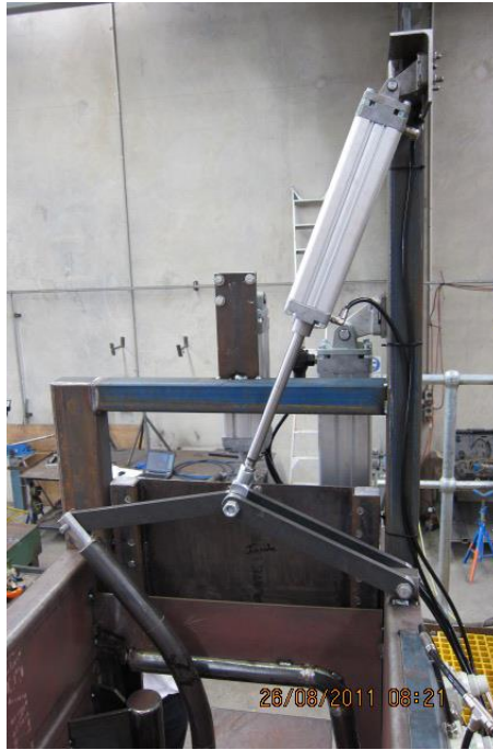
Figure 4 - Cylinder device in position to operate the head bale. Site visit to G & B Stainless 26 August 2011.
