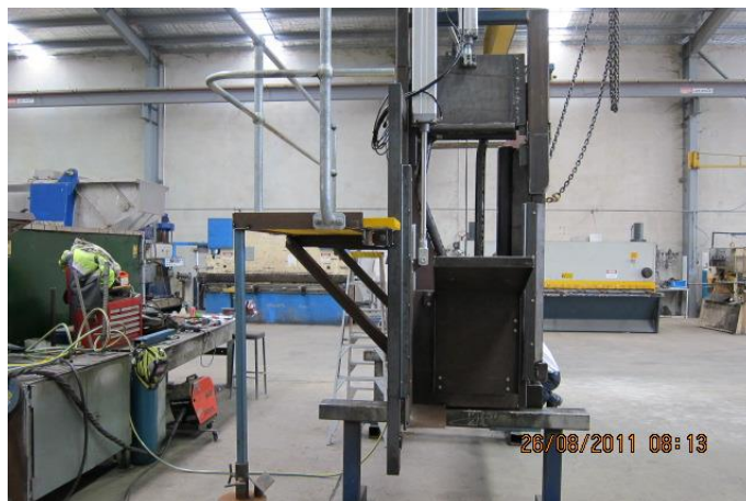
Figure 3 – The front elevation of the restraining box featuring the pneumatic cylinders for the head bale and head lift devices. Site visit to G & B Stainless 26 August 2011.
