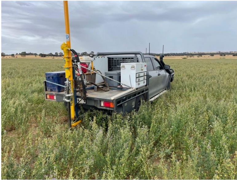
Fig. 6. 38mm soil corer used for 0-30 cm sampling (image courtesy of SYNC Agri)
