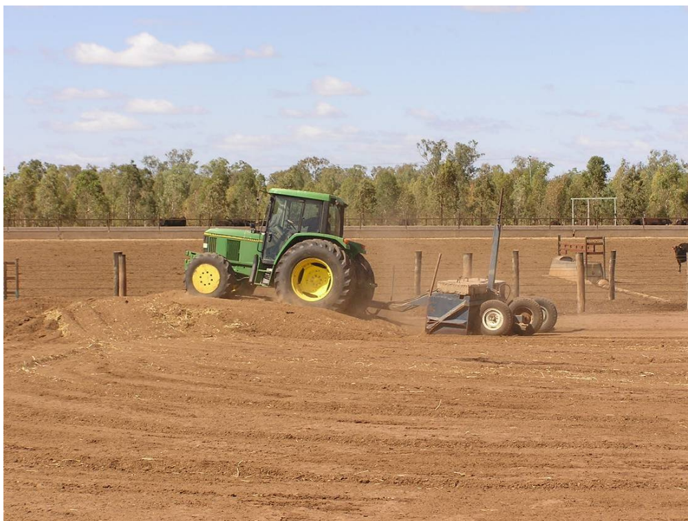
PHOTOGRAPH 3 - BOX SCRAPER USED TO CLEAN FEEDLOT PENS
