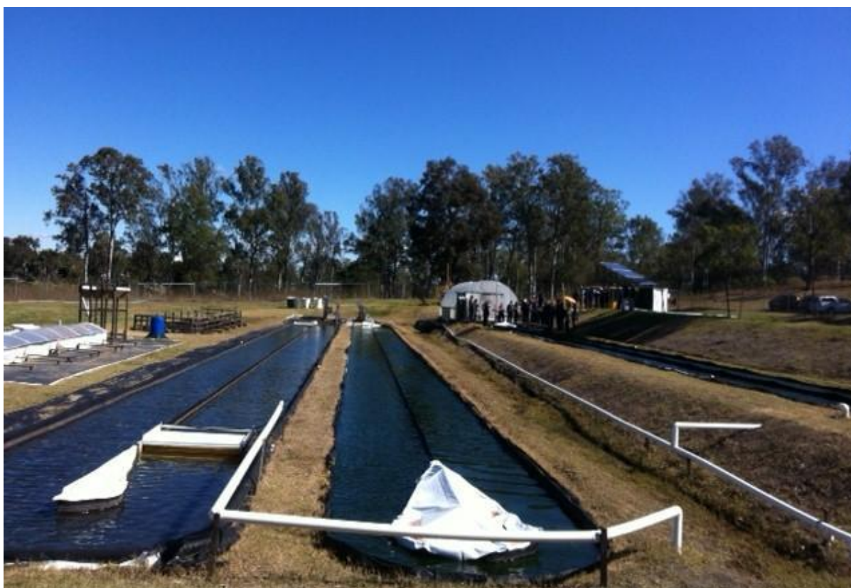
Fig. 3. Cultivation of Scenedesmus dimorphus NT8c in raceway ponds (in July 2014).
