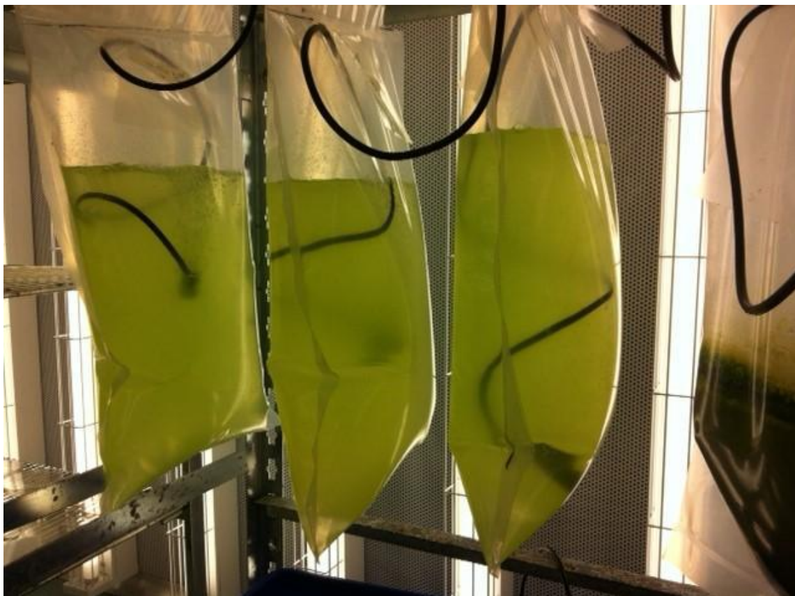
Fig. 5. Scale-up of cultivation in 10 L bags in the laboratory before culturing outdoors
