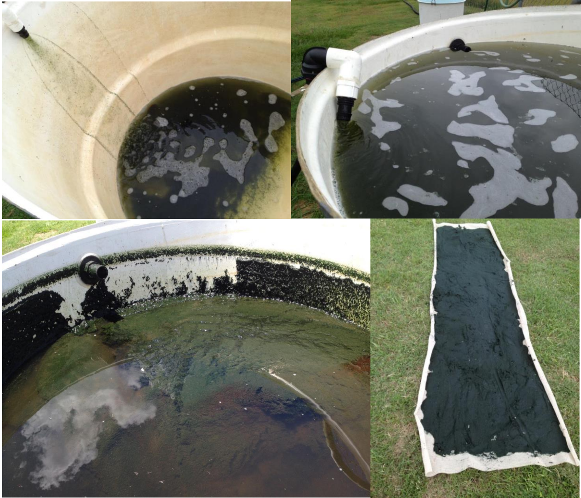
Fig. 27. Automated continuous harvesting system developed for Limnithrix using settling in 1000 L tanks. Shown are the start of filling up a 1000 L tank, the 1000 L tank once filled to the overflow, the collected sludge after 2 x 12 h runs, and secondary dewatering via draining onto shade cloth.
