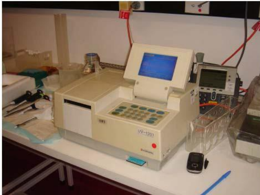
Figure 14: Detection Equipment: Shimadzu UV-1201 UV/VIS Spectrophotometer for measuring light absorbance.
