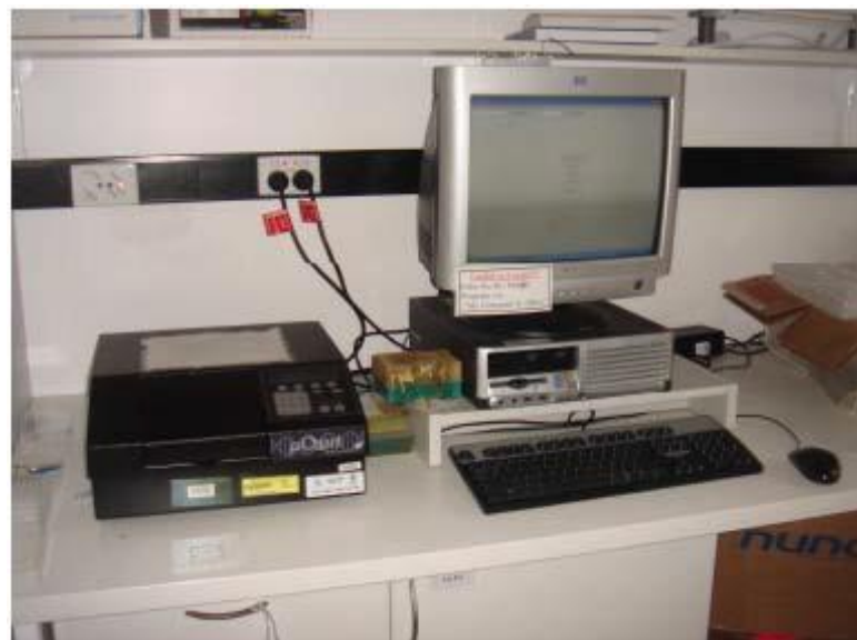
Figure 13: Detection Equipment: Biotek uQuant microplate spectrophotometer for 6, 12, 24, 48, 96 and 384 well plates e.g. for ELISA assays of AP activity.
