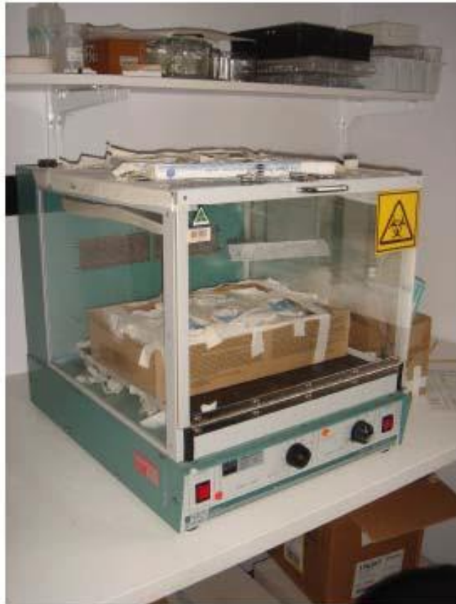
Figure 11: Temperature controlled cell incubator.
