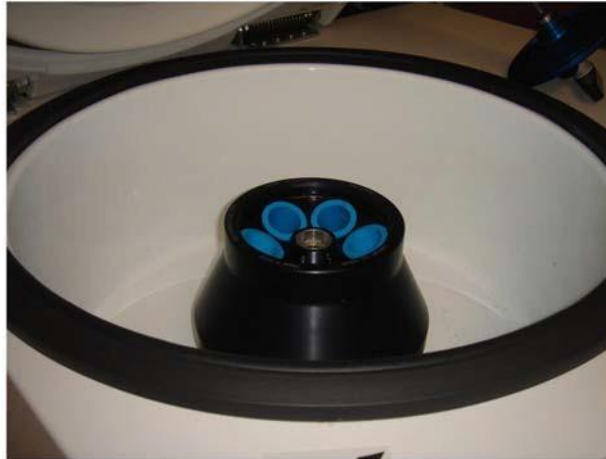
Figure 6: Rotor for processing 5 x centrifuge tubes.
