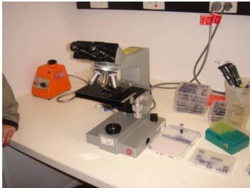
Figure 12: Microscope for cell counting (centre) and vortex for cell re-suspension (left).
