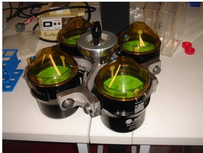
Figure 5: Rotor bucket for processing 16 x centrifuge tubes simultaneous.
