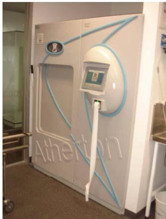
Figure 15: Autoclave for sterilizing equipment.
