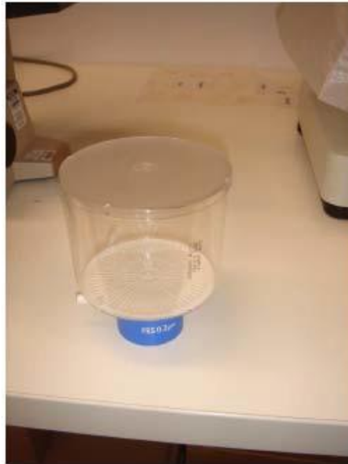
Figure 7: 0.2 micron filter for sterilizing liquids.
