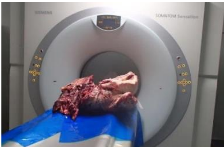
Figure 9 - Beef quarter prepared for Helical CT scanning.
