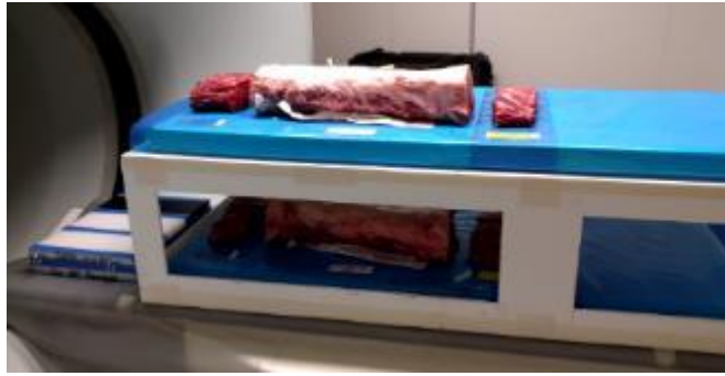
Figure 89 - Scanning arrangement for striploins
