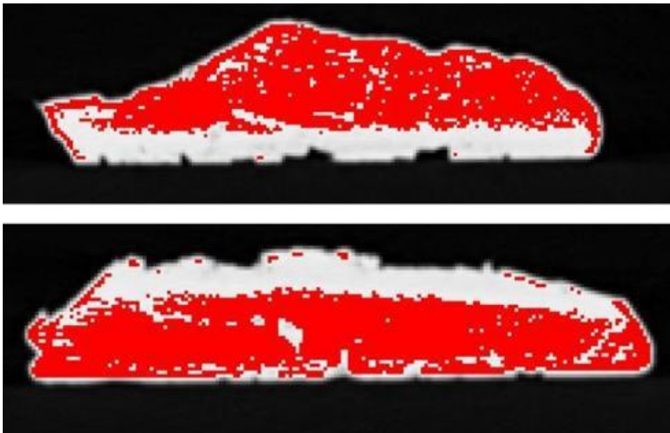
Figure 7. Computer tomography images showing low density pixels (<1077 units) in white.
