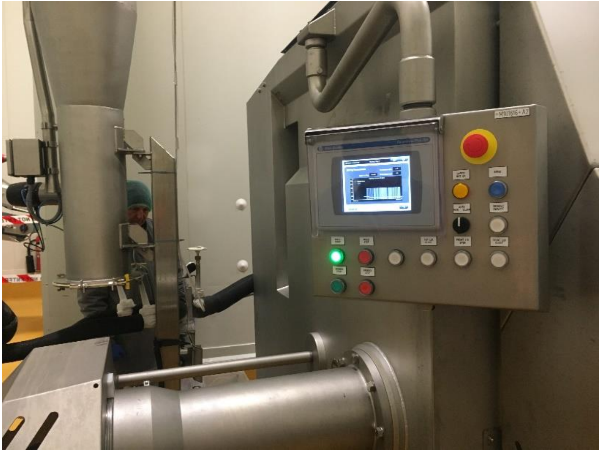
Photo 6: Mixer interface screen used for monitoring cooling cycle
