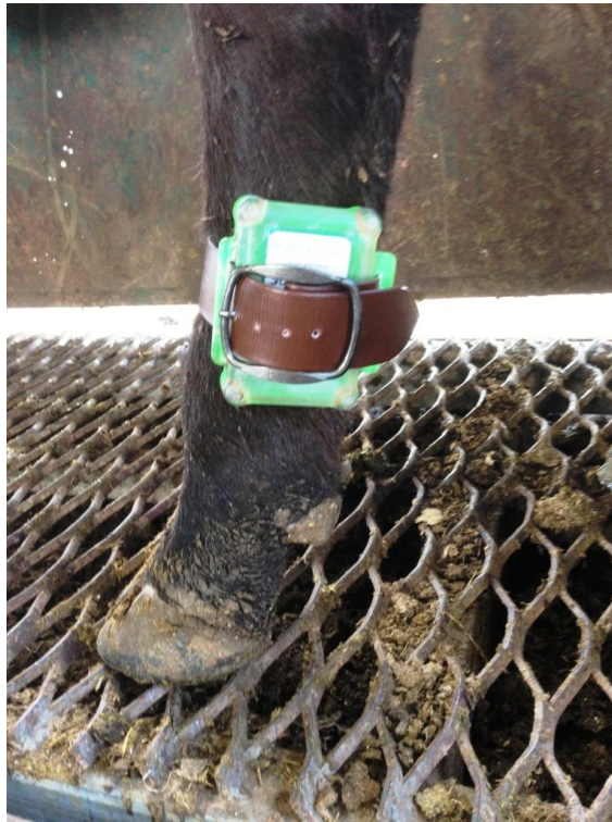
Figure 4. Ictag devices attached to the hind leg of cattle, used to remotely measure lying and standing behaviours.
