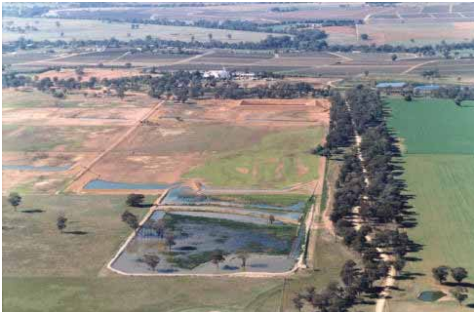
Effluent irrigation showing wet weather dam, irrigation area and flooded woodlot
