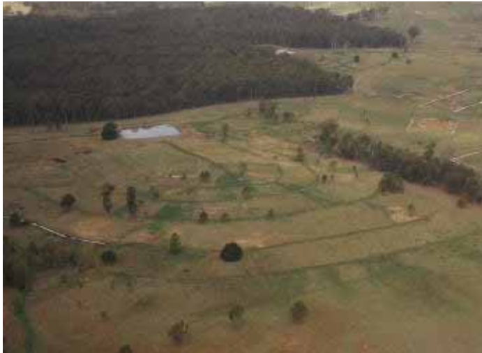
A flood irrigation scheme showing contours to direct effluent
