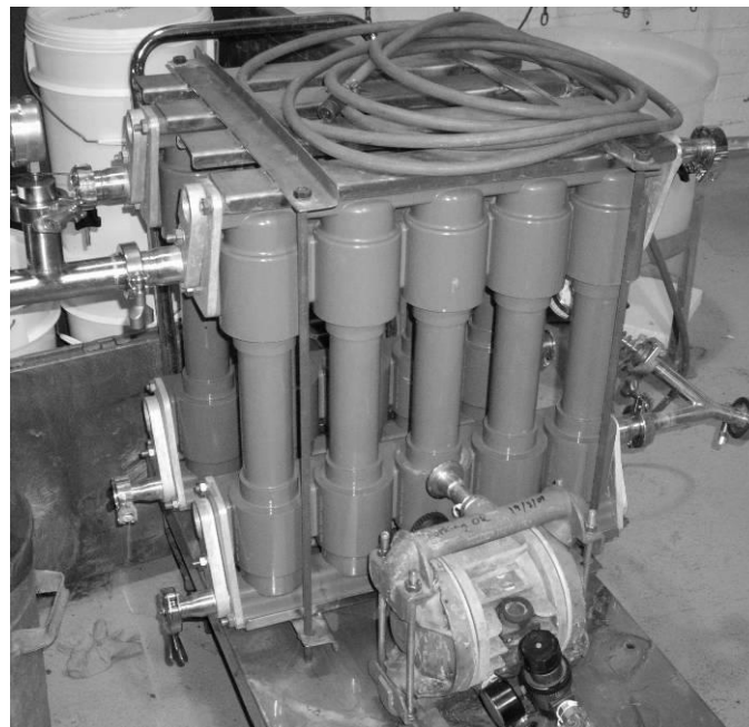
Figure 9: MEMTEC bank of hollow fibre membranes. The diaphragm pump shown below is used to provide pressure.
