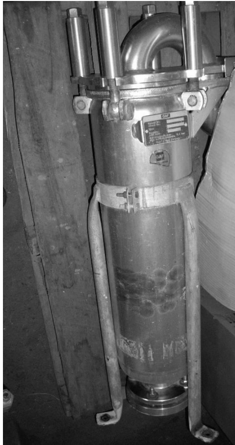
Figure 8: GAF filtration setup. A bag held in place by a stainless steel mesh is placed inside the filtration apparatus.
