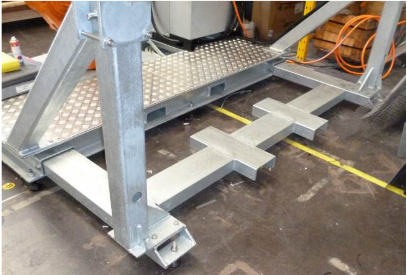
Fig.1 Retractable conveyor base supports
