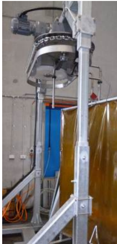
Fig.2 Conveyor posts that can be lowered for transport
