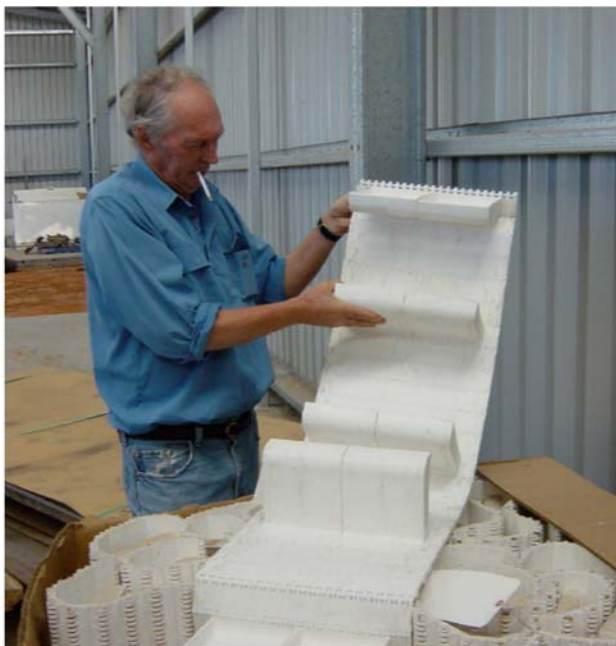
Photograph 5 - Anton Reiter demonstrating the flexibility of the Intralox belt
