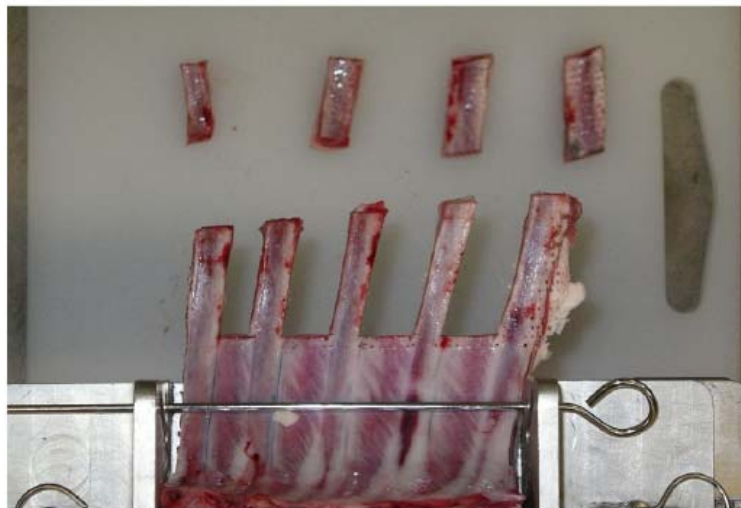
Figure 1 – Multiple knife configuration. Results demonstrated that this approach is effective.
