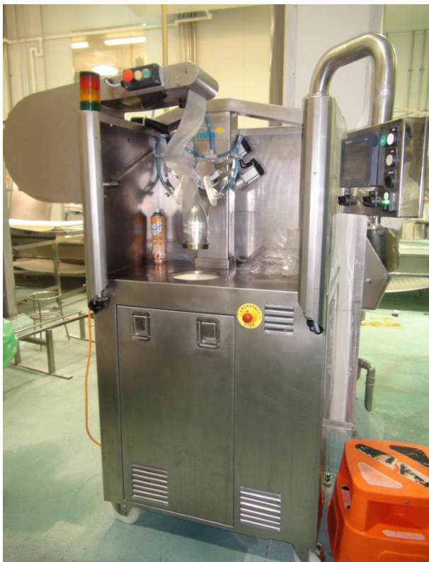
Figure 7a,b: Step 3: Packaging secured and ready for product to be loaded.
