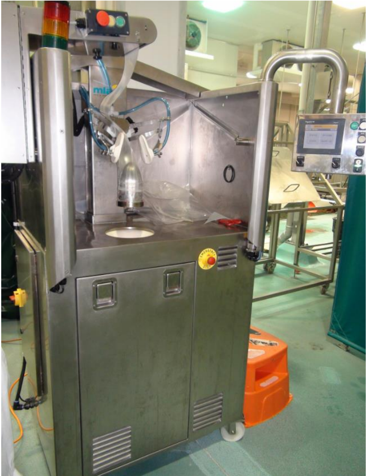
Figure 4. MLA's existing (FixAll Services) SmartShape prototype featuring a new auto-bagging option
