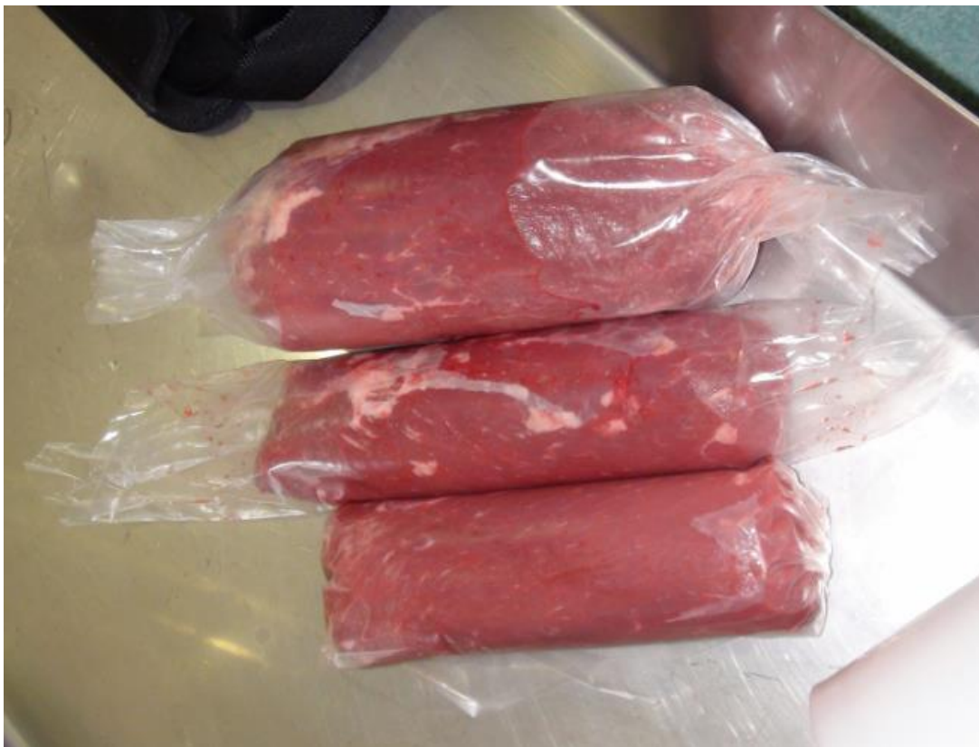
Figure 9: Step 5: Packaged product removed from SmartShaping machine ready for clipping.
