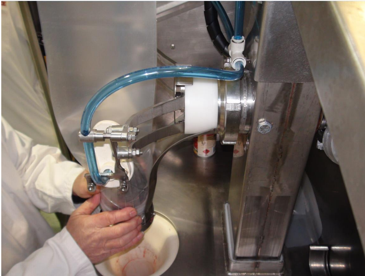
Figure 6: Step 2: Bag fed onto filling mechanism.
