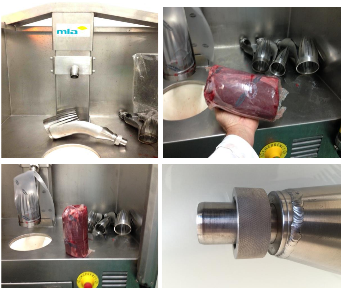
Figure 13: New bag holder design
