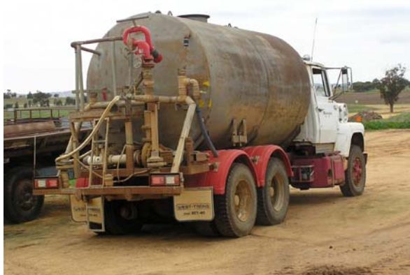
Photograph 20 - Water truck for road maintenance and dust suppression
