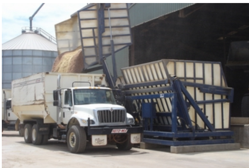
Photograph 13 - The Batch box System incorporates a side dump box
