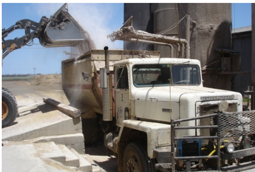
Photograph 12 - Screw mixer feeder loaded with commodities by a front-end loader
