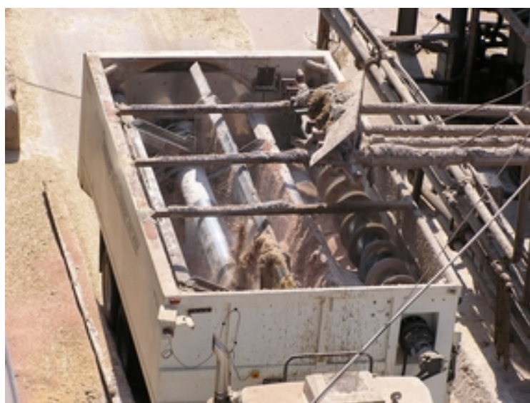
Photograph 11 - Truck mounted 920 -18 'Roto-mix' mixer feeder
