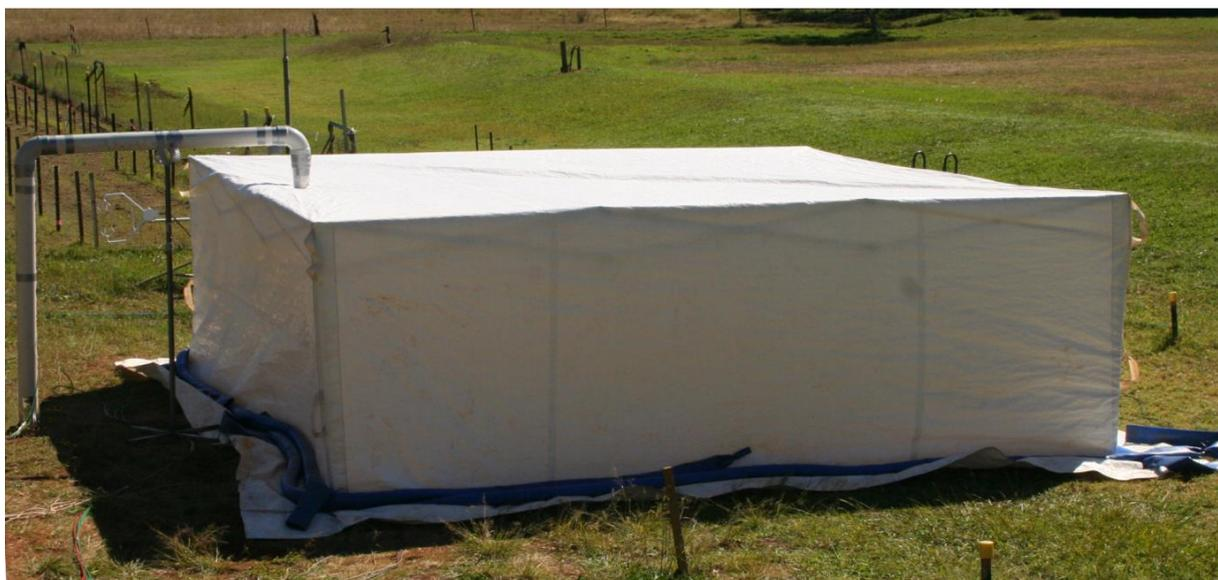
**Figure 2.2.** The fabric covered large chamber is based around a modified commercial gazebo (4.5 x 4.5 x 1.5 m high) covered with a polyethylene-coated fabric.
