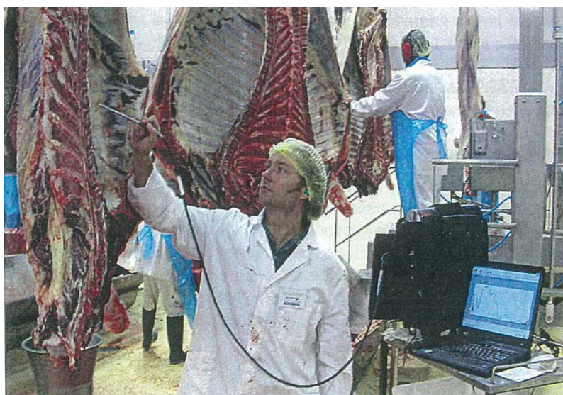
Figure 1 Beef carcass loin muscles being measured with the ASD multi wavelength spectrometer fitted with a fibre optic probe on the slaughter floor operating at 90 —95 carcasses per hour.
