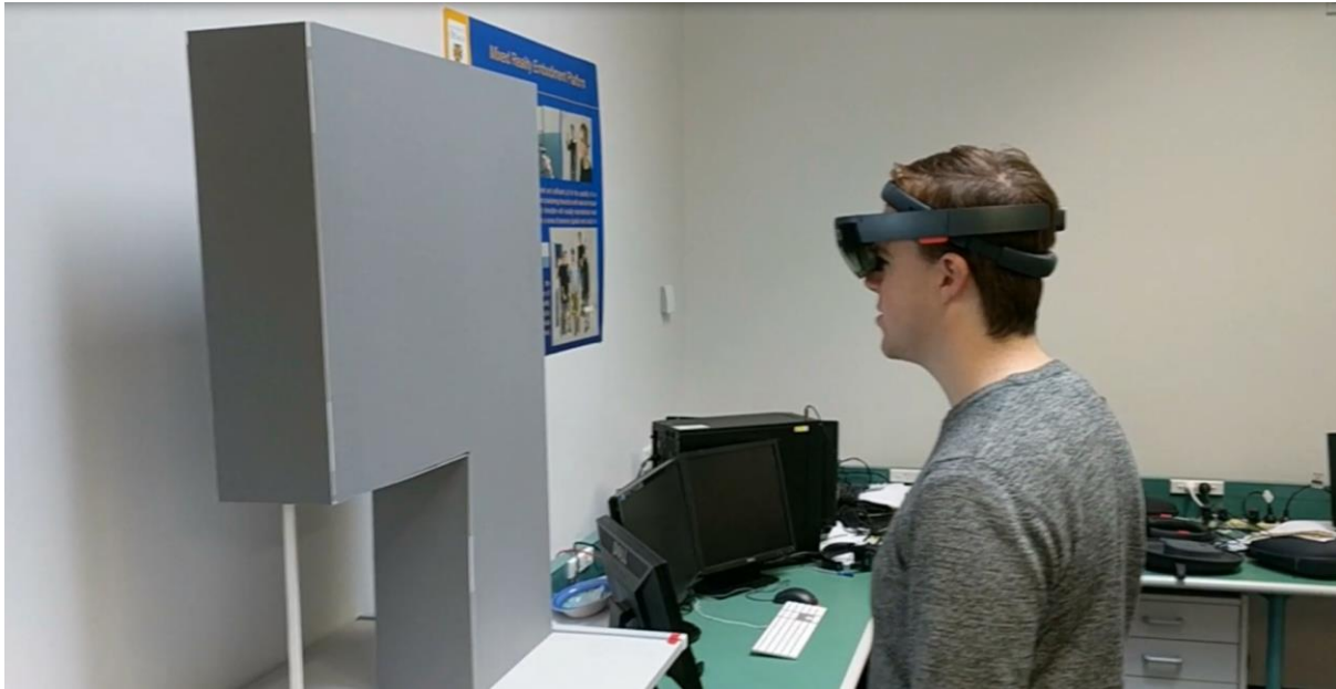
Fig. 1: A Hololens-wearer approached a mock-up Bladestop bandsaw.
