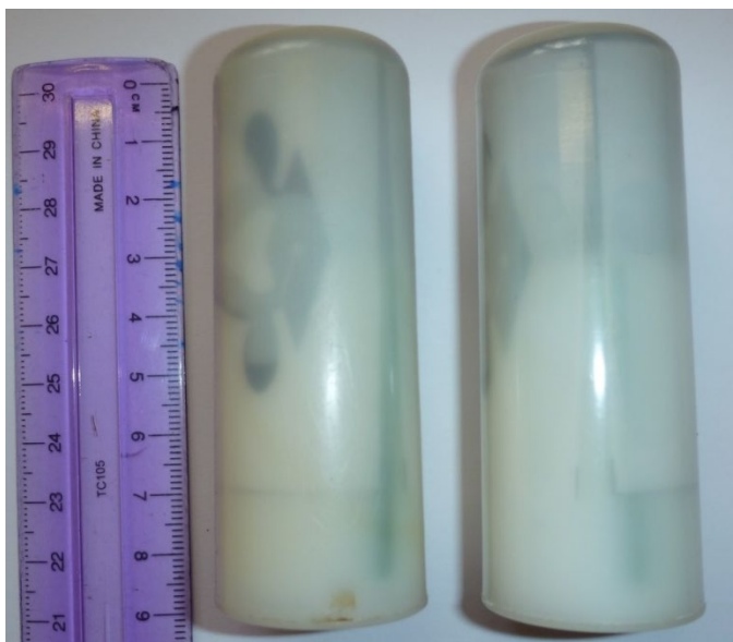
Figure 2 A new bolus on the right and a recovered bolus on the left.
