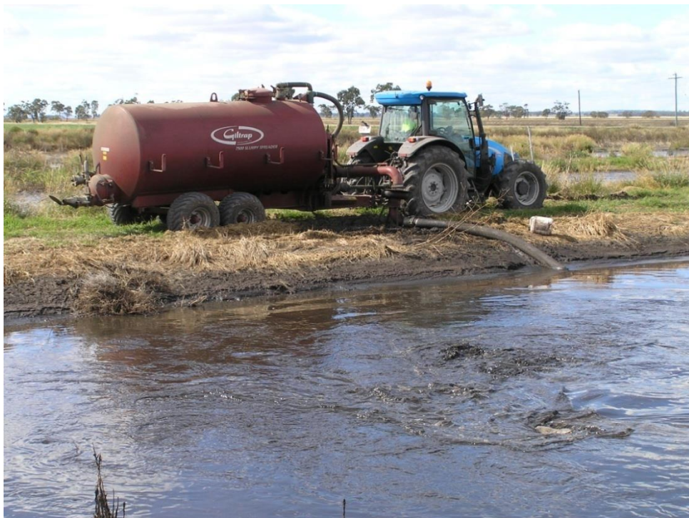
PHOTOGRAPH 10 – SLUDGE REMOVAL USING A SUCTION TANKER AND AGITATION (SOURCE: ALAN SKERMAN, DAFF)
