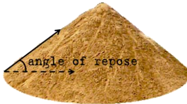
FIGURE 8 – SCHEMATIC DESCRIPTION OF ANGLE OF REPOSE
