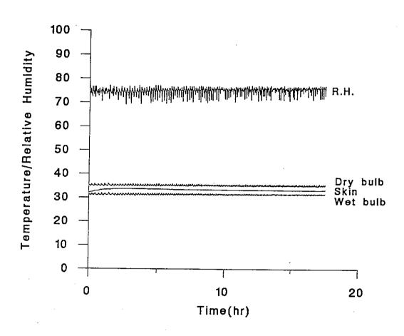
Fig. 2. A typical recording of dry bulb temperature, wet bulb temperature, skin temperature and calculated relative humidity during an overnight incubation.
