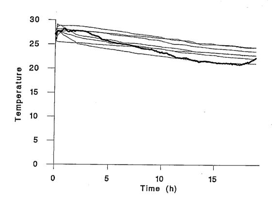
Fig. 16. Time/skin temperature profiles obtained with acetate buffer preserved skins during the abattoir trials. The heavy line is the ambient temperature.
