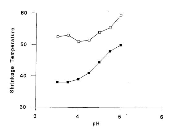
Fig. 19. Shrinkage temperatures of (■) soaked and (□) painted skins measured at the paint pH.
