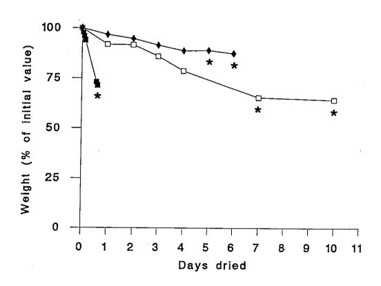
Fig. 8. Time course of weight loss and ease of depilation for skins dried in air during (■) summer, (□) winter or in a (♦) 4°C chiller. (★) indicates difficult depilation.
