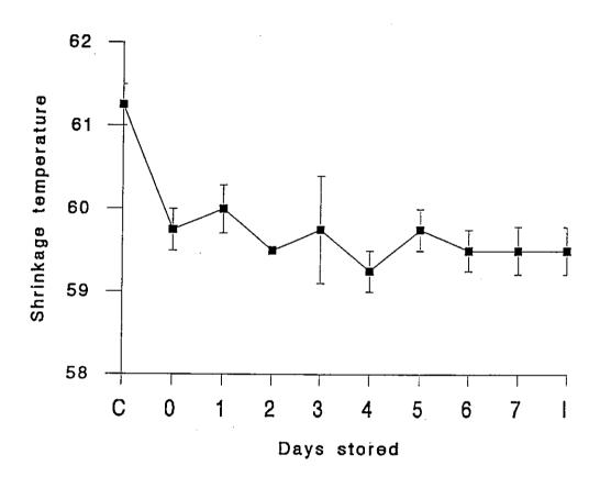
Fig. 15. The average shrinkage temperature (n = 4) obtained with samples of acetate preserved skins after various storage times. For comparison the values obtained with pre-painted (C) and post-incubated skin (I) are included.
