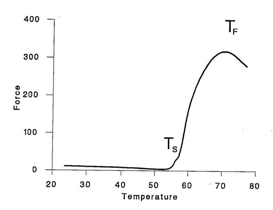
Fig. 1. Measurement of the shrinkage  $(T_s)$  and failure  $(T_p)$  temperatures.
