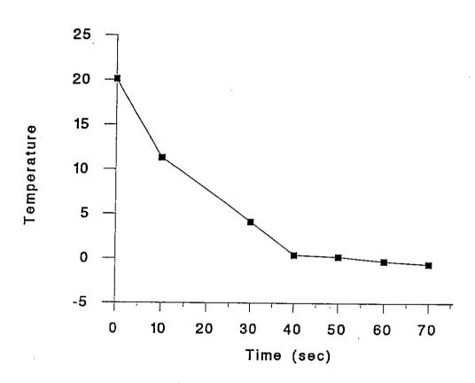
Fig. 11. Dependence of chilled skin temperature on the time on the plate freezer.
