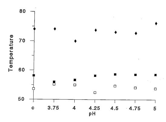
Fig. 18. Effect of depilant pH on the thermal stability of fellmongered and pickled skins. ( $\blacksquare$ )  $T_s$  of skins, ( $\square$ )  $T_s$  of pelts and ( $\blacklozenge$ )  $T_F$  of pelts (c) control.
