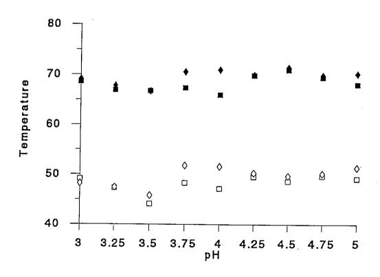
Fig. 20. The effects of acetic acid concentration and pH of the depilant paint on the  $T_s$  (open symbols) and  $T_F$  (closed symbols) of pickled pelts. The acetic acid concentration was ( $\blacksquare$ ) 40% or ( $\spadesuit$ ) 20%.
