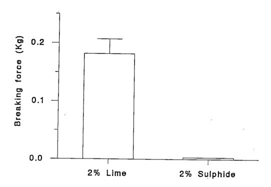
Fig. 22. The effects of exposure of wool to lime or sulphide prior to lime/sulphide treatment.
