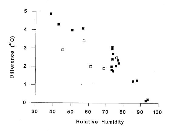
Fig. 24. The effect of humidity on the difference between dry bulb and skin temperatures. Dry bulb temperatures were ( $\blacksquare$ ) 35°C or ( $\square$ ) 30°C.
