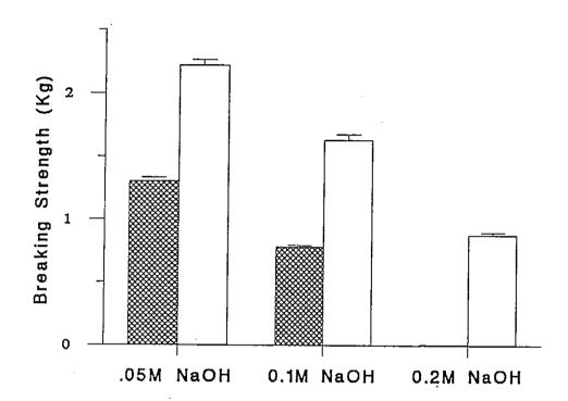
Fig. 21. Effect of 1% (v/v) (hatched) or 0% (plain) mercaptoethanol on the breaking strength of wool in the presence of differing concentrations of NaOH.
