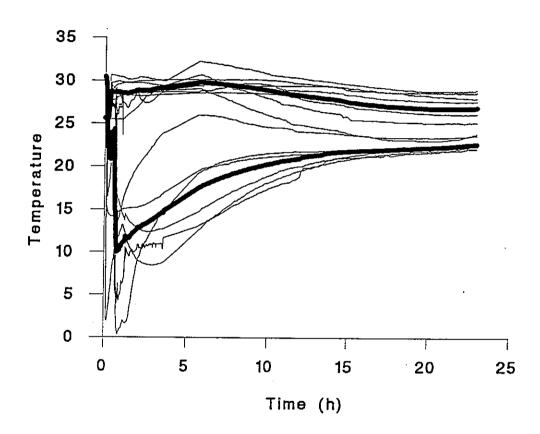
Fig. 13. Typical skin temperatures versus time plots obtained during the abattoir plate freezer trials. The lower six traces were for chilled skins and the top eight traces for untreated skins. The heavy lines are the averages.
