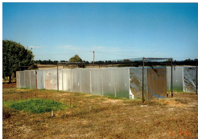
Figure A9.1. Temperature gradient tunnel imposing CO 2 and temperature treatments as described by Lilley et al. (2001). Photograph J. Lilley.
