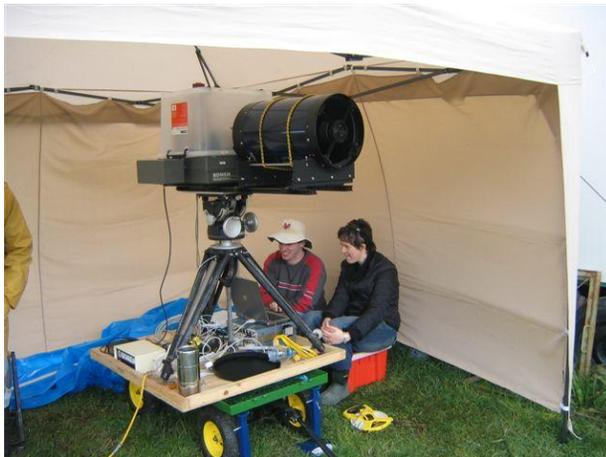
**Plate 1:** Open-path Fourier Transform Infrared (OP-FTIR), including Bomem spectrometer, in the field at Feedlot A.
