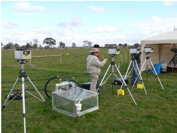
**Plate 2:** Open-path lasers in the field at Feedlot A.
