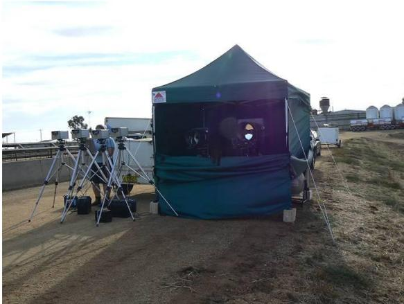
**Plate 3:** Side by side calibration of OP lasers and OP-FTIR, including Bruker spectrometer, in the field at Feedlot A.
