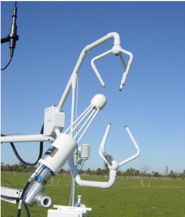
**Plate 5:** Detail of three-dimensional sonic anemometer and infrared gas analyser on micrometeorological station.
