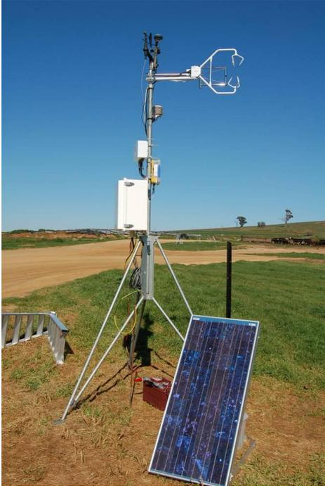
**Plate 4:** Micrometeorological station in the field at Feedlot A.
