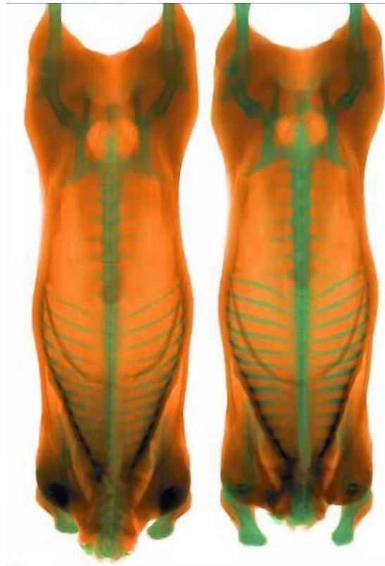
Figure 1. A NUCTECH DEXA scan (high and low energy images) of a standard lamb carcass captured on-line at Wagstaff Meats.
