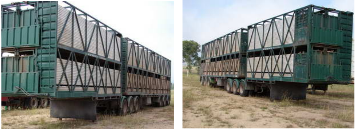
Figure 4. Two views of a typical well-used B-double livestock transport crate. This one includes walk-through loading, airbag suspension and steel and alloy construction incorporating extruded aluminium sideboards. Loading may be either side or rear, with side loading making for easier vehicle positioning before loading/unloading
