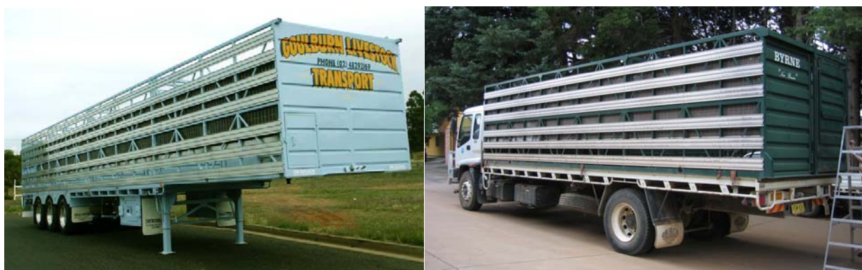
Figure 3. Left: Photograph of a semitrailer unit for livestock transport, convertible between one deck for cattle and two decks for sheep, with four internal pens. Right: Fixed body tray truck fitted with a 3 pen x 1 deck crate for cattle, convertible to 3 x 2 for sheep
