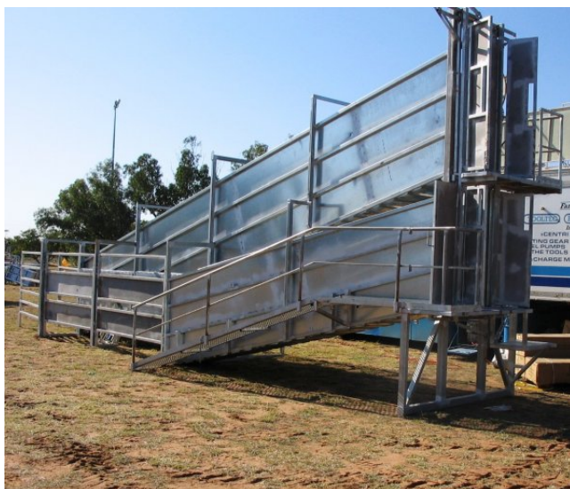
Figure 7. Photographs of double deck loading ramps. The animals are either directed into the right-hand race (which curves inwards to become the lower ramp), or straight ahead to the upper loading ramp. The structure running up the left-hand side of the ramp on the right is a catwalk for stockpersons to assist with loading. These ramps are made by Towers Engineering of Charters Towers in Queensland.
