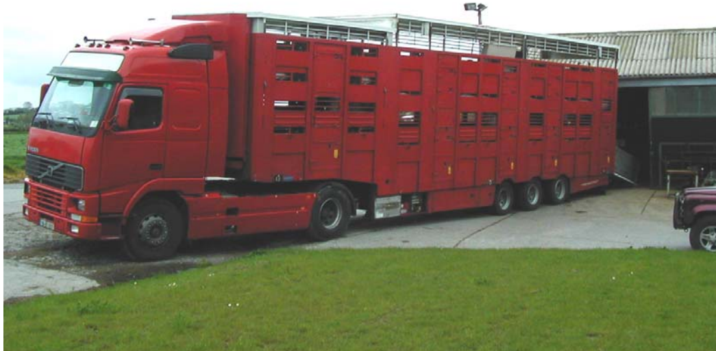
Figure 6. Photograph of a long-haul European transport vehicle. Note the adjustable ventilation flaps, some of which are covering electric fans for forced ventilation. Another aspect to note is the drop-down loading ramp at the rear, which loads animals from ground level. The vehicle is convertible between one and three decks, with decks being raised by hydraulic rams once loaded. There are three internal pens, and an on-board water supply and water drinkers.
