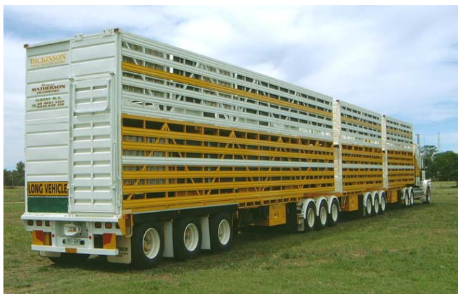
Figure 5. 4 x 2 convertible B-Triple unit with walk-through rear loading, hydraulic internal ramp winch and spring suspension
