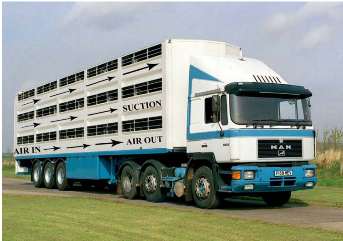
Figure 1. A European livestock transport vehicle illustrating the direction of natural ventilation. Some crate designs used in Australia have comparable ratios of solid walling to open areas, although Australian vehicles have more air inlets at the level of the feet of the animals, which may provide better air movement under Australian climatic conditions and reduce humidity build up from moisture from faeces and urine on the deck.
