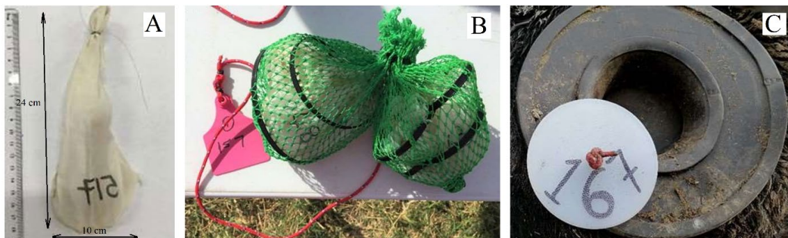
Figure 3.7. (A) Numbered polyester bag folded and secured with fishing line prior to application of a rubber band; (B) Two sets of biopolymer pieces within set bags containing weights and showing zip tie spacer rings, nylon rope and initial ear tag used to secure through the rumen canula, and (C) Solid disc securing bags through the rumen canula.
