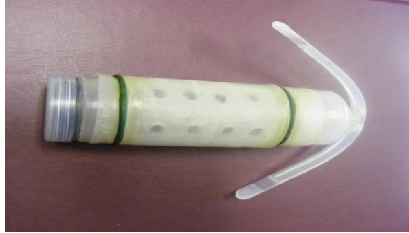
The inter-rumen gas measuring device. Source: CSIRO
