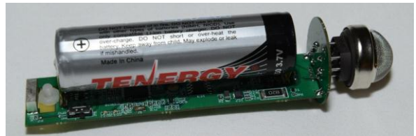
The battery and sensor equipment. Source: CSIRO
