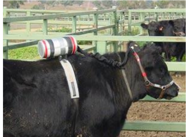
A steer being measured for methane production: NSW DPI
