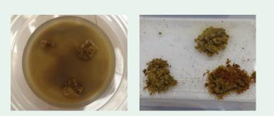
Pictured: Cloudy water indicating dispersion of soil crumbs; collapsed crumbs indicating slaking.
