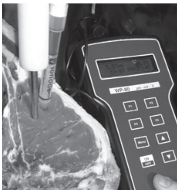
ENSURING MSA QUALITY STANDARDS ARE MAINTAINED, WE INTRODUCED AN ELECTRONIC MONITORING SYSTEM FOR 114 COMPANY GRADERS. (PH MEASUREMENT PICTURED HERE)
