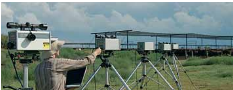
Measuring ammonia from a feedlot using an open path laser.
