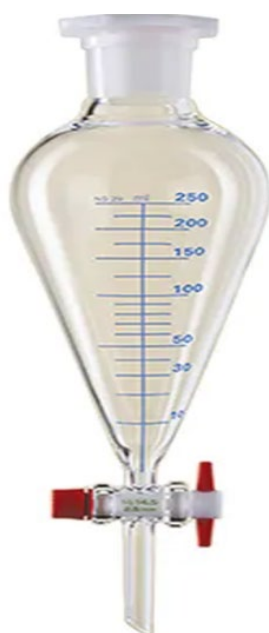
Figure 12. Glass squib used to hold liquid supplement treatments
