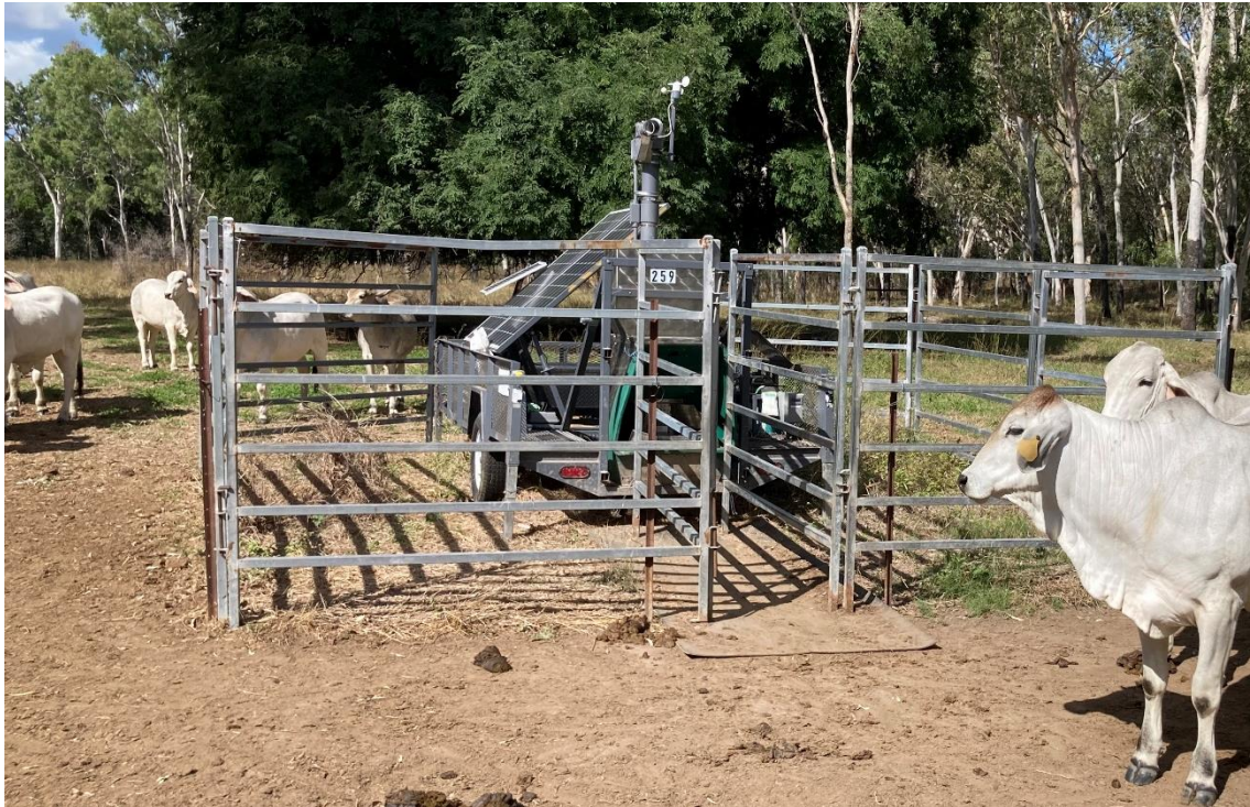
Figure 3. Gas emissions monitoring (GEM) unit deployed for long-term monitoring of methane from grazing cattle.
