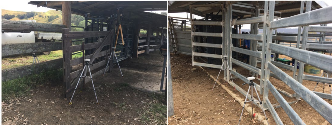
Figure 3. Standard flight time testing setup.
