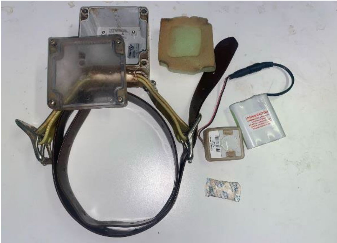
Figure 29. Image of GNSS collar and components used on both commercial properties during the study.
