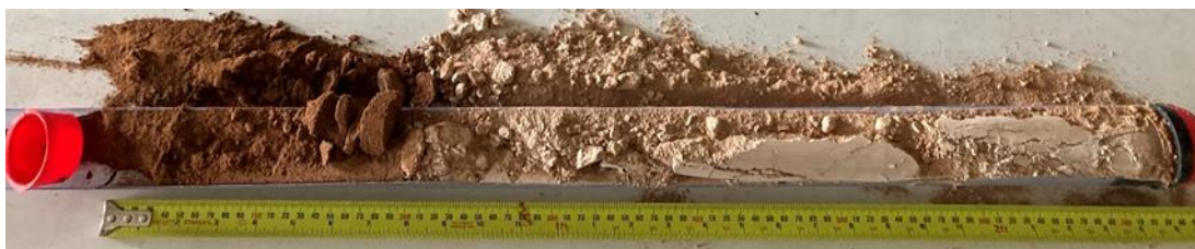
Figure 125. Profile 28048 from Pooncarie Region (Property #7 Site 2, stratum 4). This soil had a sandy surface and visible carbonates from 30 cm. The carbonates were mainly soft with some hard nodules. While not evident, the upper profile displayed effervescence of the fine-earth fraction indicating the presence of carbonates
