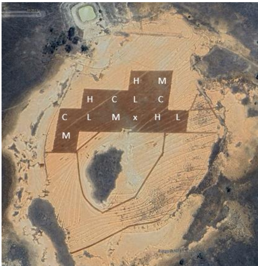
Figure 22. Satellite image of Gurrawarra Gypsum site following incorporation of gypsum and location of treatment replicates (C = control/nil gypsum, L = low rate 1 t/ha, M = moderate rate, 2.5t/ha, H = high rate, 6.5t/ha. Site x was avoided due to an adjacent sand mound). Banks were established around the site to minimise run-on
