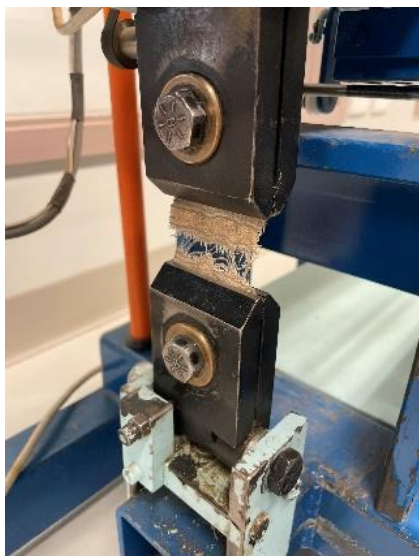
Figure 32. Piece of cotton strip being tested for tensile breaking strength in the tensometer
