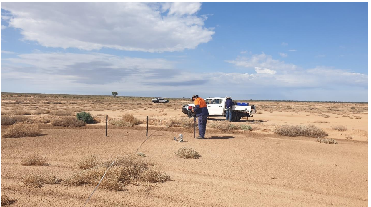
Figure 19. Soil sampling in March 2024. Three cores were sampled parallel to the ponding bank at 5m and two-thirds of the distance of the pond to the spill points
