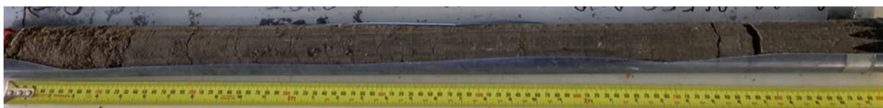
Figure 126. Profile 26550 from the Brewarrina region (Property # 3, Site 2, stratum 2). The heavy soil from a drainage area had low salt content. There was only a small abundance of carbonate nodules from 15 cm increasing below 25 cm though still <2% from a visual estimate
