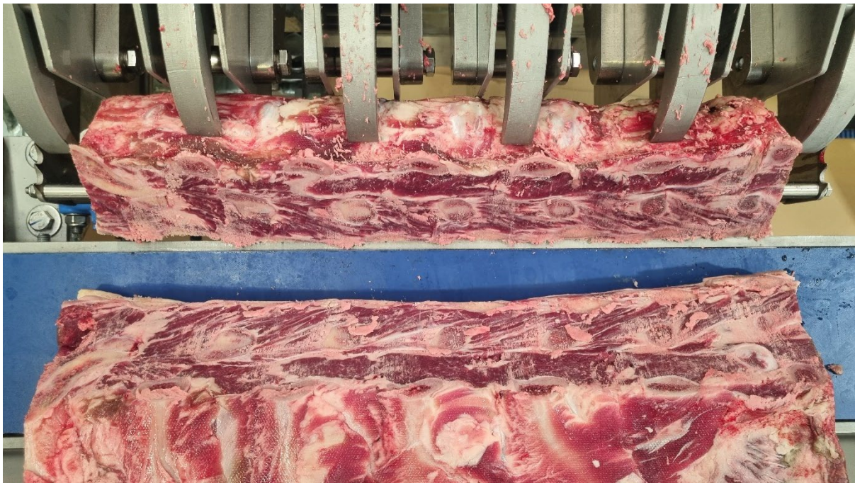
Figure 13 – SL9, chine bone still clamped, showing bases of button bones, feather bones and transverse processes.
