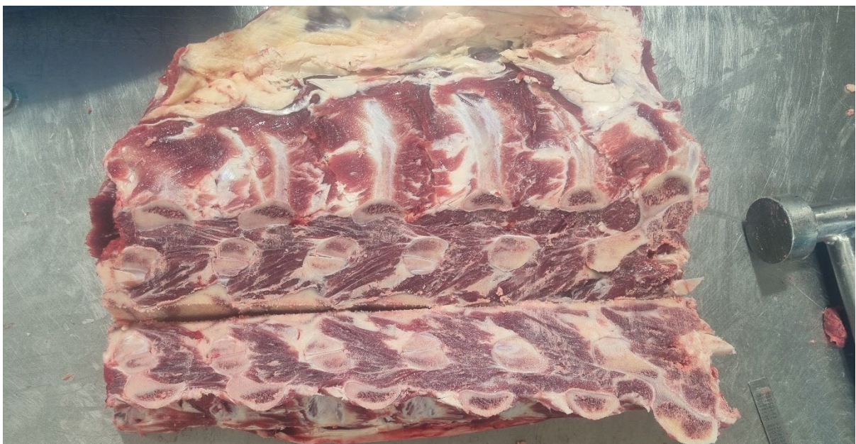
Figure 30 – Example of striploin with chine bone as cut by robot bandsaw.
