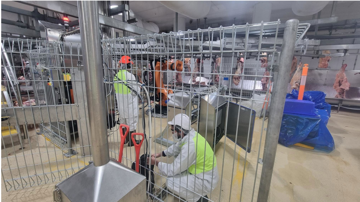
Figure 25 – Robot being re-mastered & vision system being commissioned.
