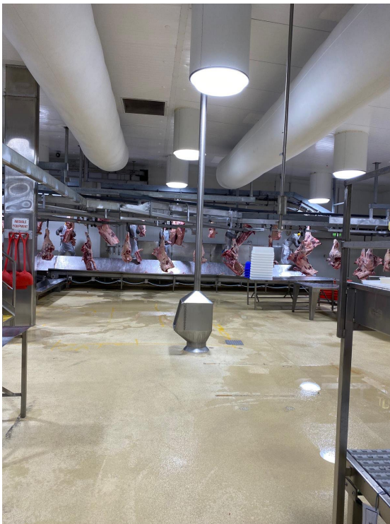
Figure 21 – Room preparation works: Meat rail above robot cell removed & belt conveyor cut back.
