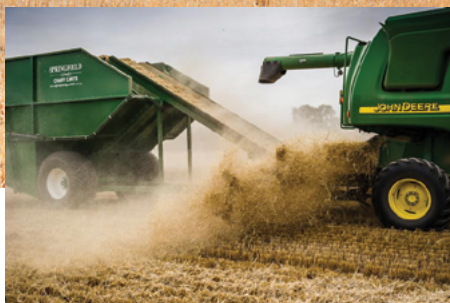
Wheat chaff heaps (above), collected using a chaff cart towed behind the harvester and dumped in rows (right). Credit: Dr Dean Thomas from springfieldgrenfell.com.au
