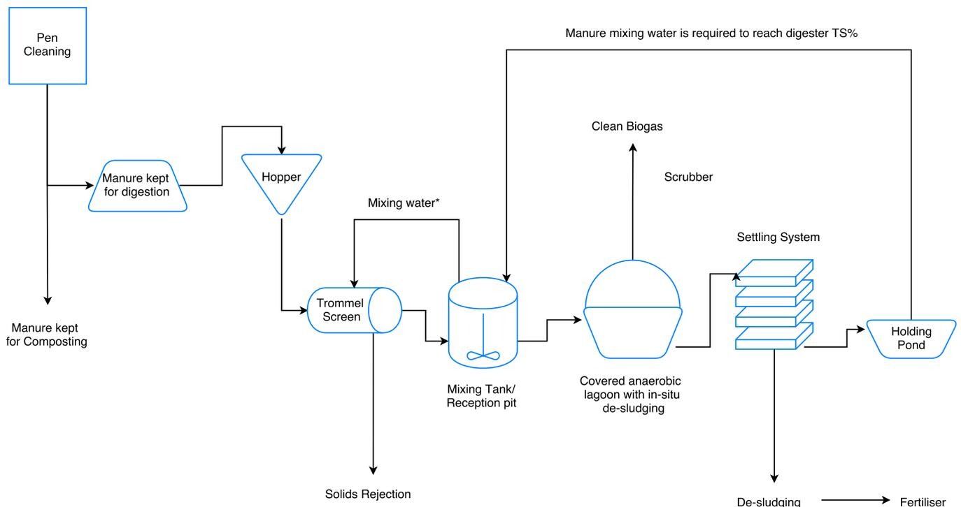
\*Mixing water is used as a water jet to remove debris from Trommel screen and further break up manure before entry mixing tank.
