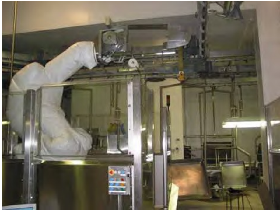
Figure 2-8 Safety Cell at Ralph's Meat Company (Note: Main control panel)
