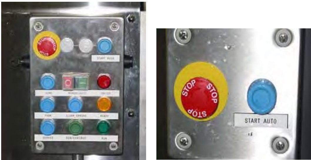
Figure 2-25: The Primary and secondary slaughter floor control panels provide the operator interface in the harsh environment of the slaughter floor
