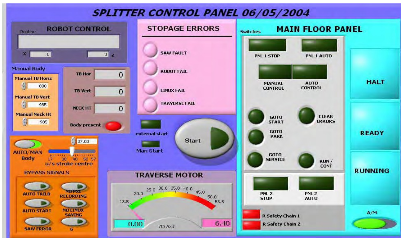
Figure 2-29: Technical user interface for the main PXI control unit
