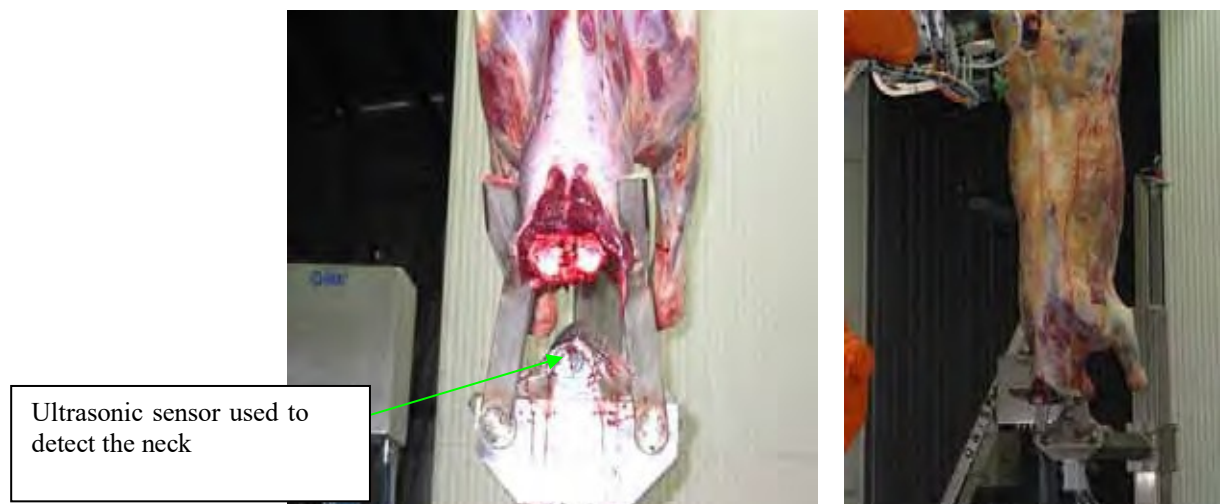
Figure 2-17: The neck stretcher in place showing the ultrasonic sensor used to detect the bottom of the carcass and the jaws pulling the carcass down during the cut
