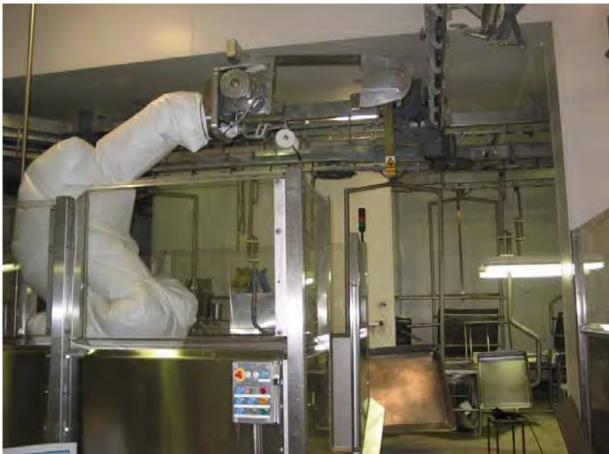
Figure 2-26: The primary slaughter floor control panel is located at the exit of the safety cell
