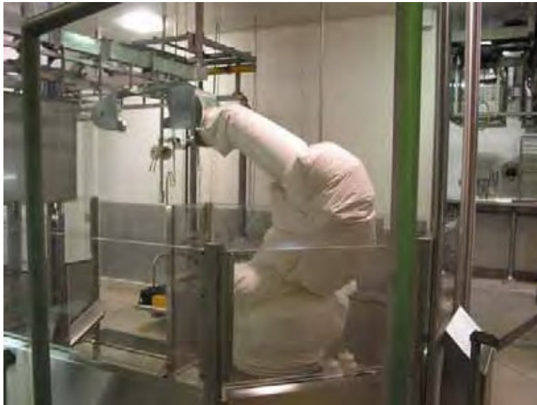
Figure 2-20: Automatic splitting system installed at Ralph's Meats in a category 3 safety cell.
