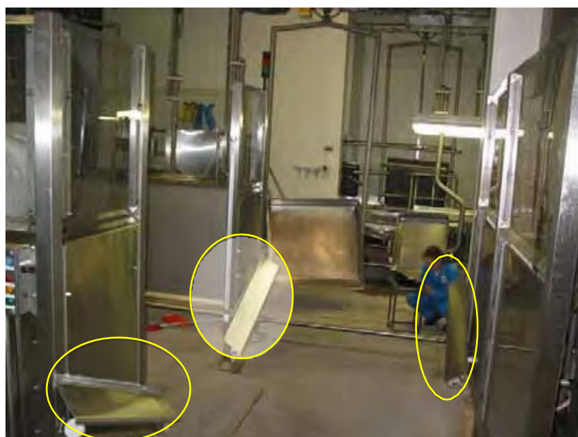
Figure 2-24: The safety cell entry is protected at entry and exit by light curtains
