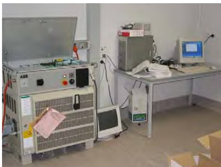
Figure 2-28: Inside the control room electronic components could be protected from the harsh environment of the slaughter floor. Later the screen and keyboard for the PXI controller would also be located in this room
