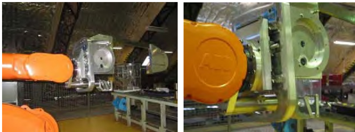
Figure 2-13: The traverse motor controlled the movement of the saw from side-to-side and was part of the robot end-effector
