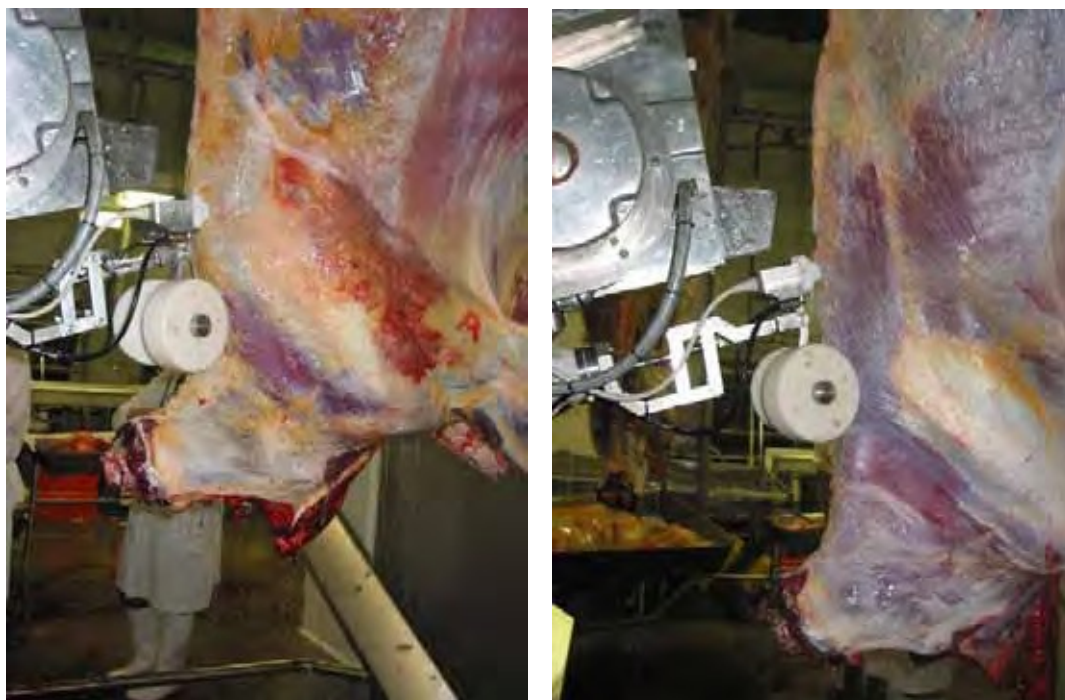
Figure 3-14: Water sprays were fitted below the ultrasound head to wet the carcass surface
