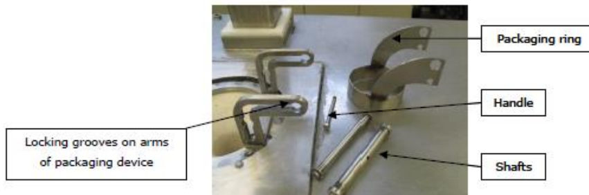
Figure 7. Packaging device disassembled
