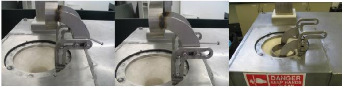
Figures 6a, b & c. Packaging device locked in upright position, unlocked position and locked in rubber sleeve ready to receive meat sample
