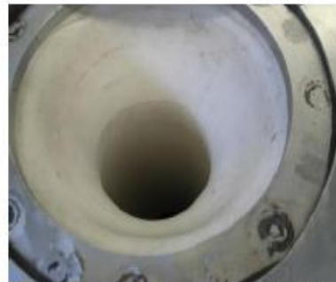
Figure 2b. Rubber sleeve expanded to allow insertion of meat sample
